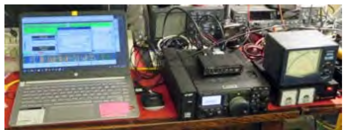
Equipment as used at PCARA's 2023 Field Day VHF station. L to R: HP notebook, Yaesu FT-897D, SCU-17 interface, Daiwa CN-801 output meter and DC power supply.
