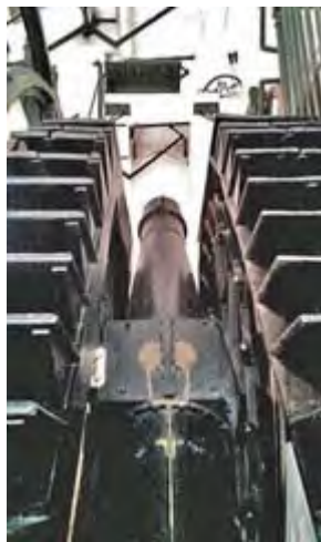
Airy’s transit circle telescope at Greenwich allowed observation of time and angle above the horizon as stars cross the meridian. [Credit: CCA 2.0]
