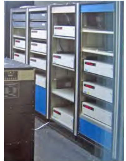
Racks of cesium beam atomic clocks at the U.S. Naval Observatory in Washington DC help provide standard time for the Department of Defense and the entire U.S. [Credit: USNO]
