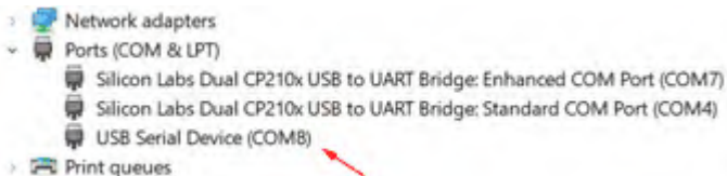
Windows Device Manager “Ports” section shows two COM ports assigned to FT-991A followed by COM8 (arrowed) assigned to HiLetgo satellite receiver.
