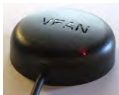
VFAN magnetic puck has a small red LED that blinks during satellite reception.
