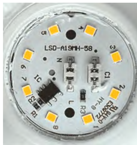
Karl's teardown of a 60 watt Sylvania soft white LED bulb revealed this PC board. [N2KZ pics.]
