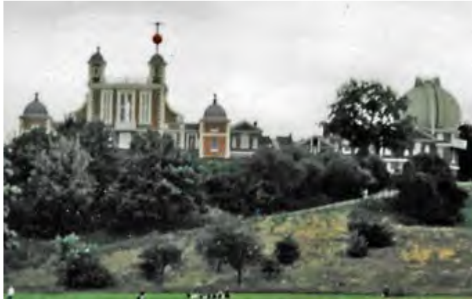
The Royal Observatory, Greenwich stands on a hill overlooking the River Thames in southeast London. Lowering of the red time ball on the tower at exactly 1:00 p.m. indicated Greenwich Mean Time to nearby ships. [G3VNQ 2000 pic.]
