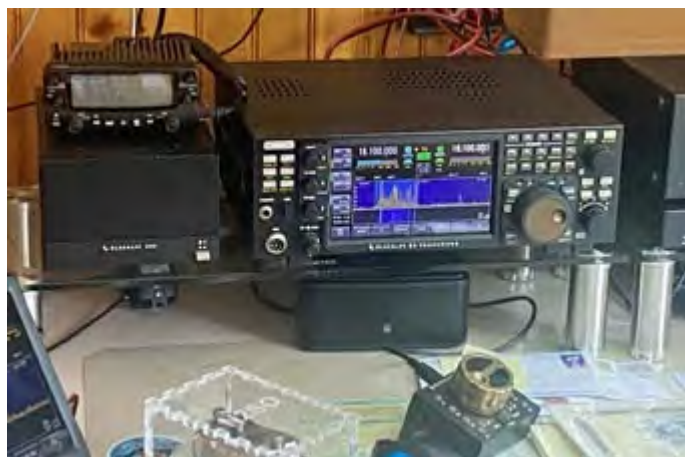
Elecraft SP3 speaker, Elecraft K4 transceiver, and (below) Elecraft K-Pod external control panel. [KD2WSU pics.]
