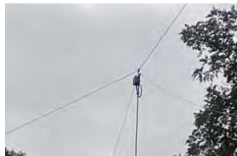
Off-center fed inverted-V dipole has feed-point suspended by 'messenger' line.
