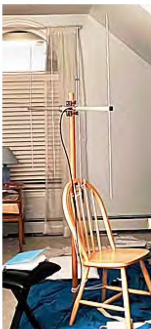
4-Element Yagi antenna with chair support at N2KZ. [Credit: N2KZ]
