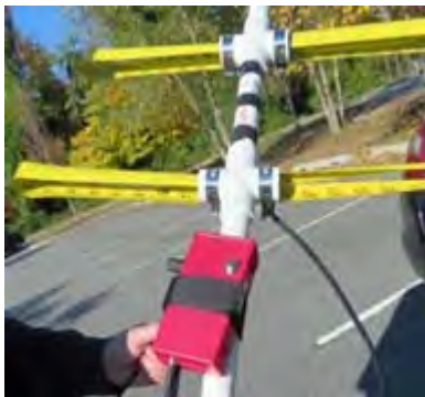
Rob AD2CT had an offset active attenuator for his antenna.
