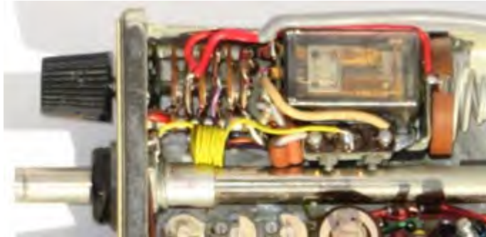
Transmit/Receive relay is mounted behind the Off/Volume/Mute-off rotary switch. Mechanical switch below the relay transfers RF output from coaxial connector to the telescopic rod antenna when this antenna is fully extended.
