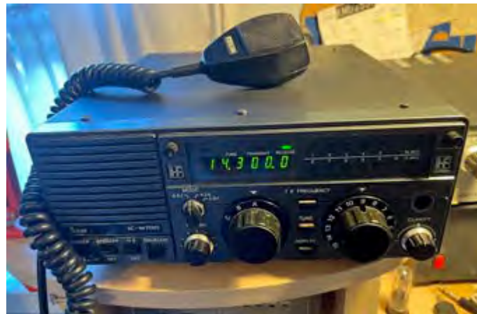
Icom IC-M700 150 watt SSB transceiver recently acquired by Todd N2MUZ covered marine bands from 1.6 MHz to 22.9999 MHz. [Pic credit: Todd, N2MUZ]
