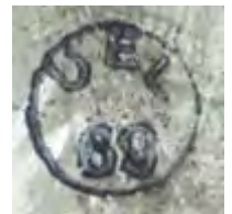
Mark on zinc-plated steel chassis ‘UEL 69’.
