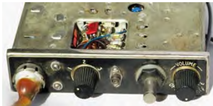
Ultra Electronics low-band FM transceiver had (L to R) mic connector, three channel switch, miniature coaxial antenna socket, telescopic antenna and Off/Volume/Mute-off rotary switch.
