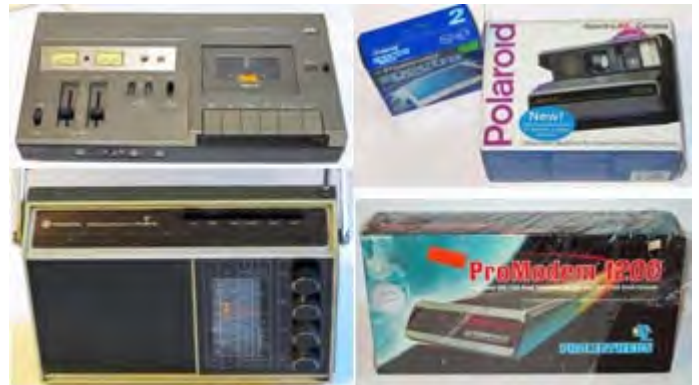
Four more items from the ‘Shelf of History’. A JVC stereo cassette deck with Dolby noise reduction, a Polaroid Spectra instant color camera with film pack, a WH Smith Multiband receiver covering LW, MW, Marine Band (1.6-4.4 MHz) and two SW bands – and a Prometheus ProModem 1200 dial-up modem, vintage 1984.
