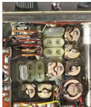
Crystal sockets and trimmer capacitors inside the low-band radio. Crystals for 6746.66 and 5855 kHz had been fitted.
