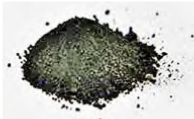
Powder form of lithium iron phosphate is grey or black.
